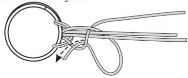
Step 4d: Pull both long cords to slide the first half of the square knot up tight.
